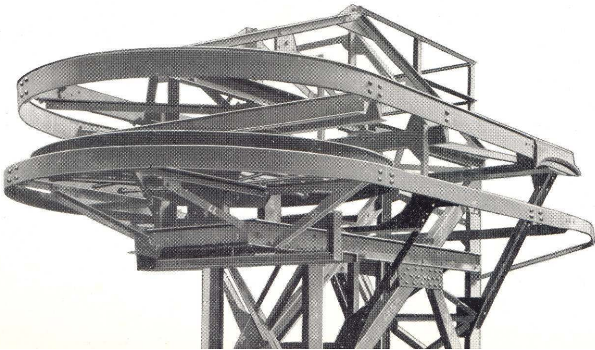
AERIAL ROPEWAY STATION complete with pulley fabricated and assembled to customer's design and specification.
